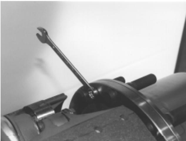
**Picture 2.** Unscrewing hub housing retaining screws.
