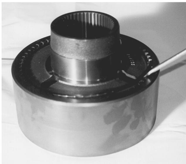
**Picture 8.** Retaining ring removal.
