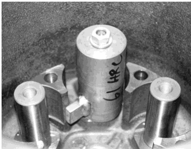
**Picture 5.** Planet gear shafts removing with a special tool.
